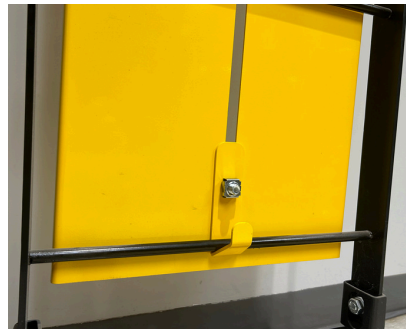
Step 2. Adjust and tighten the lower hook
